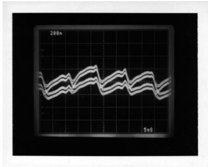
Figure 4.8. Eye pattern at 100 Mbps for a 2^7-1 PRBS with the oscilloscope triggered on every fourth bit.
